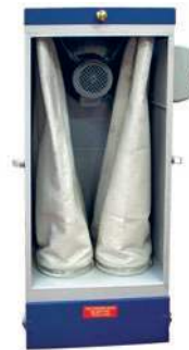
Inside a F41 Dust Collector
