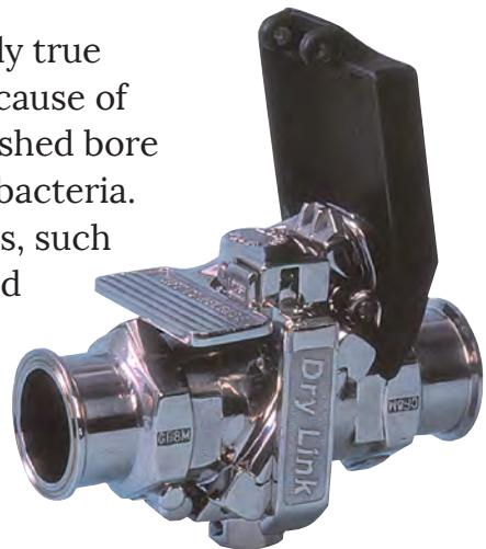
Dry Link sanitary couplings are usually specified with wetted internal components polished to 20RA micro-inch mirror finish. Wide choices of sizes, body and seal materials and end connections with full material test certifications. MTR, FDA and USP certifications are available.
